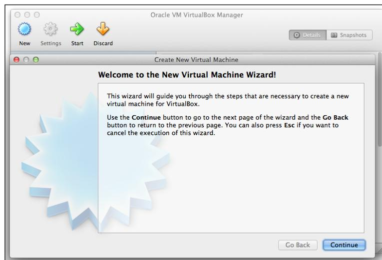
You will be asked to enter a name and OS type on the next screen. Next, select the memory to allocate for the VM. The recommended base memory size is 192 MB. The next screen asks you to either create a new disk or use an existing disk. When installing a new OS from a disk or image, you will want to select **Create new hard disk**. On the next screen, use the already selected default, **VDI** (VirtualBox Disk Image), and then select **Dynamically Allocated**.
